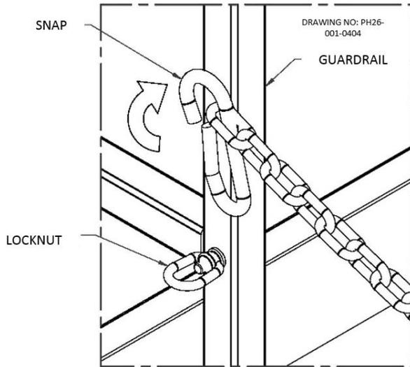
1. Disengage the chain hook from the guardrail eye nut to enter or exit the platform
